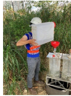
Installation of Mariotte Bottles
